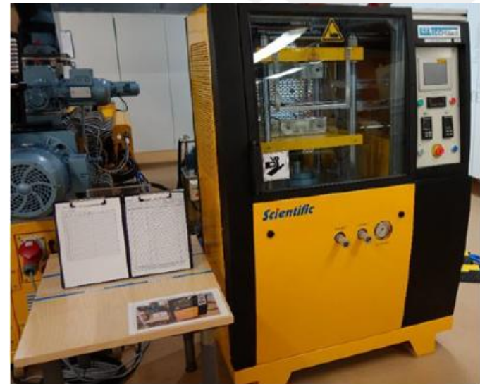
Compression moulding with Hydraulic thermoforming press: Labtech Engineering LP-S-20
