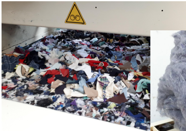
Sorted fibres cut to pieces in two directions
