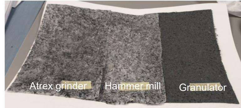
Foam formed sheets from shortend fibres
